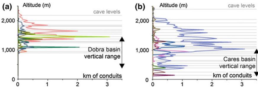
**Fig. 4** **a** Vertical distribution of conduits density of the spring catchments related to Dobra basin. **b** Vertical distribution of conduits density of the spring catchments related to Cares basin
