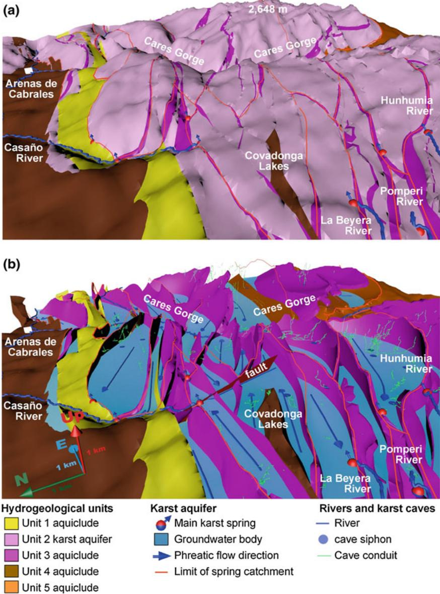
**Fig. 2** a Zoom on the hydrogeological model showing the limits of the main karst springs catchment. The position of the point of view is displayed in Fig. 1. b Same view excluding the volumes of limestone (karst aquifer) in order to display the groundwater bodies (saturated aquifer), phreatic flow directions, and documented caves conduits and siphons
